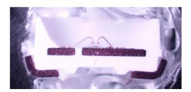
17. Defendants' M670 Series also includes a platform covering said first opening, said platform being located outside said aperture, with a light emitting diode mounted on the platform within the aperture, and a transparent encapsulant material encapsulating the light emitting diode in the aperture:
