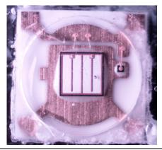
38. Defendants' 3535 Series also includes an LED having a metallized bottom major surface that is mounted on the electrically conductive mounting pad, the metallized bottom major surface comprising one of an anode and a cathode of the LED:
