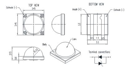
37. Defendants' 3535 Series also includes an electrically conductive mounting pad located on one of the major surfaces of the substrate:
